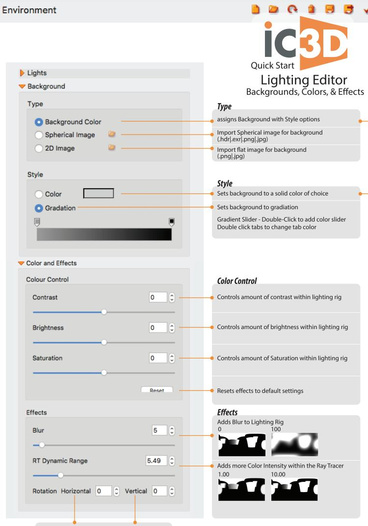
Rotates lighting rig by Horizontal and Vertical axis
